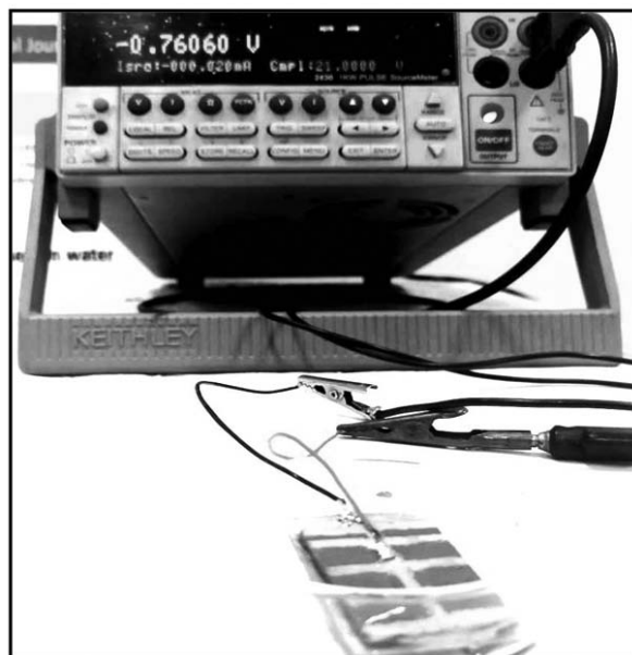
Figure 1. Experimental set-up for measurement of V-I polarization of hydroelectric cell (HEC is at the bottom).
