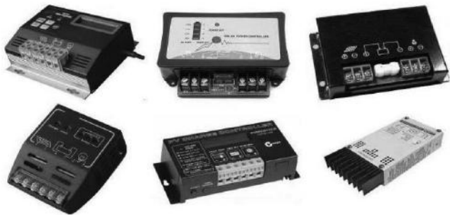
Figure 2c. Solar Charge Control llers.
