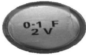
Figure 8: A coin type cell supercapacitor [27].
